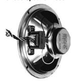
The Dukane Model 5A606 Speaker Assembly shall be an 8-inch (20.3 cm), 8-ohm, seamless cone type and shall meet the following specifications: the ceramic magnet shall weigh at least 4.8 ounces (134 g); the frequency response shall be 90 to 15,000Hz; the axial sensitivity shall be 91dB at 1 meter (3.3 ft) for 1-watt input; the normal wattage rating shall be 8 watts with a program rating of 12 watts; the
